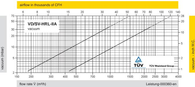
The flow capacity charts have been determined with a calibrated and TÜV certified flow capacity test rig. Volume flow  $\dot{V}$  in (m<sup>3</sup>/h) and CFH refer to the standard reference conditions of air ISO 6358 (20°C, 1bar). Conversion to other densities and temperatures refer to Vol. 1: "Technical Fundamentals".
