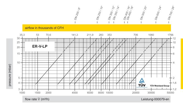
The flow capacity chart has been determined with a calibrated and TÜV certified flow capacity test rig. Volume flow  $\dot{V}$  in (m<sup>3</sup>/h) and CFH refer to the standard reference conditions of air ISO 6358 (20°C, 1bar). Conversion to other densities and temperatures refer to Vol. 1: "Technical Fundamentals".
