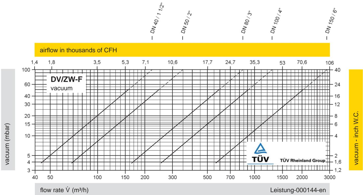
The flow capacity charts have been determined with a calibrated and TÜV certified flow capacity test rig. Volume flow  $\dot{V}$  in (m<sup>3</sup>/h) and CFH refer to the standard reference conditions of air ISO 6358 (20°C, 1bar). Conversion to other densities and temperatures refer to Vol. 1: "Technical Fundamentals".
