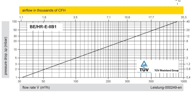
The flow capacity charts have been determined with a calibrated and TÜV certified flow capacity test rig. Volume flow  $\dot{V}$  in (m³/h) and CFH refer to the standard reference conditions of air ISO 6358 (20°C, 1bar). Conversion to other densities and temperatures refer to Vol. 1: "Technical Fundamentals".
